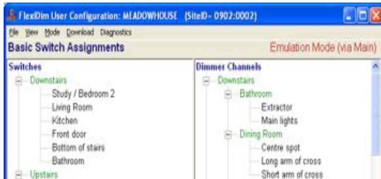
In Emulation Mode, the PC (rather than the Controllers) is receiving the button press information from Switches and sending out the commands to the Dimmer Modules.
