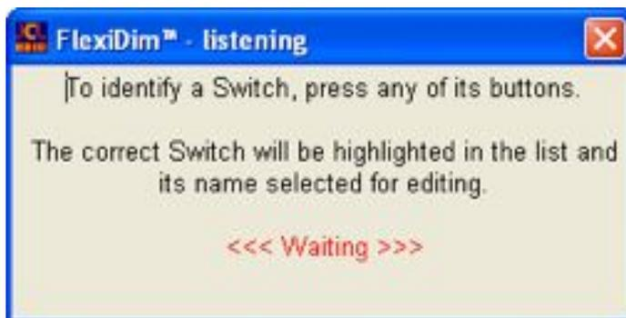
Go to the actual (physical) Switch Plate that is about to be named and press any one of its buttons in order to identify it to the Installer Configuration software.
