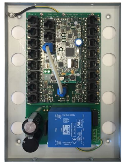
Combined Scene & Switch Controller (SC2) and Expansion Switch Controller (SW2X) (Note: Expansion Switch Controller SW2X does not have the network interface/controller boards installed)
