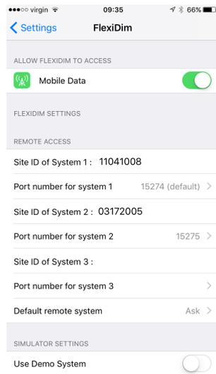
A new button has been added at the bottom of the Remote App display, allowing you to switch between local wifi or internet connection. When wifi is selected, the app will automatically connect if it can only locate one lighting system on the network, or prompt you if it can detect multiple systems. When internet is selected, the app connects to the system specified in the settings page.
